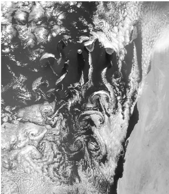
FIGURE 1. An example of a shallow wake. Aerial picture of the Canary Islands (NASA). The lower layer of the atmosphere shows typical features of a shallow flow. A von Kármán vortex street with large coherent structures downstream of the islands can be clearly seen thanks to the presence of clouds.
